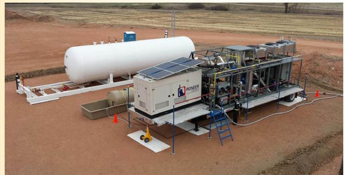
**Figure 1.** The FlareCatcher unit produces NGLs and pipeline quality methane from flare gas.
